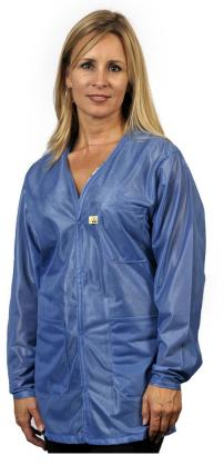
This ESD jacket is an effective Category 1 static shielding ESD garment. The lightweight OFX-100 fabric makes this style one of our most popular garments. Surface resistivity of the fabric is 1X10<sup>5</sup> and the sleeve-to-sleeve resistance of the garment is guaranteed to stay below 3.5X10<sup>7</sup> for 100 washes or 2 years.
