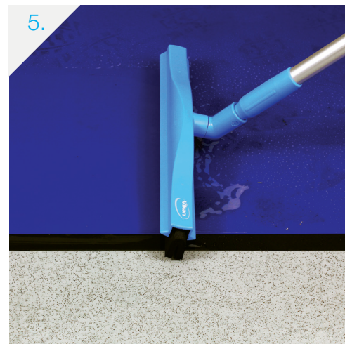
5. Agitate the Dycem surface with the squeegee in a vertical path as before, until you begin to see the contamination being lifted. Repeat this step, continuing the agitation in a horizontal direction
